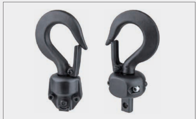
Upper and lower hooks apply material SF45C to cast which allow swiveled 360 and are equipped with safety latch to enhance the loading safety.
