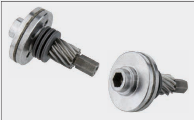
Friction clutch with lining is located outside the load patch so that the load is firmly held by brakes while hoist is disconnected from power.
