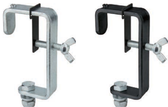
C-02N-P / C-02BN-P Clamp W 0.39kg Working Load Limit 40kg Wing Bolt / M12 Bolt & Nylon nut: yes / Protective tab: yes
