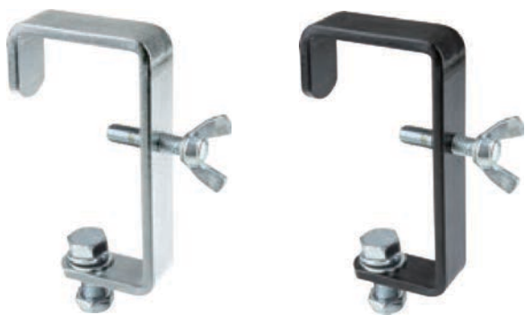
C-02N / C-02NB Clamp W 0.39kg Working Load Limit 40kg Wing Bolt / M12 Bolt & Nylon nut: yes
