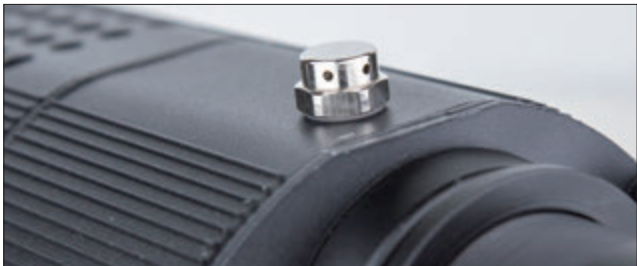
Air vent at the top equalizes the pressure and temperature, reducing water condensation and buildup inside the housing.
