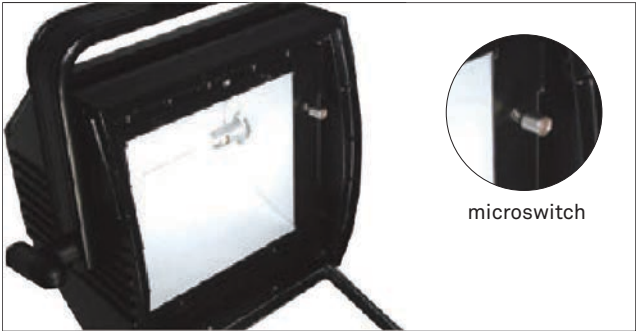
TUV Version composes the microswitch. When door is opened power of lamp housing is automatically shut off.
