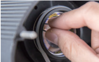
Easy to place and replace the gobo; just remove 4 fixing knobs, take off the gobo holder (a spring) and change the gobo, close the front housing, and done. That is so simple.
