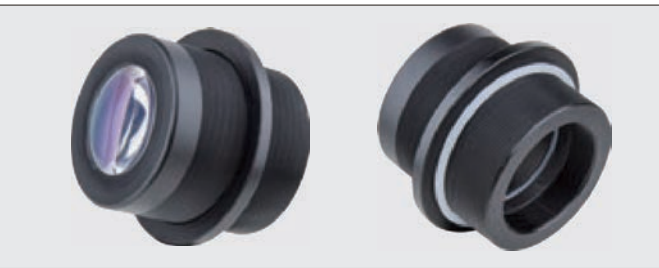
High definition optical focal lens is adjustable by turning clockwise or counter-clockwise to get the clear projection image. Make the inner ring with gasket to contact the housing firmly for waterproof seal.
