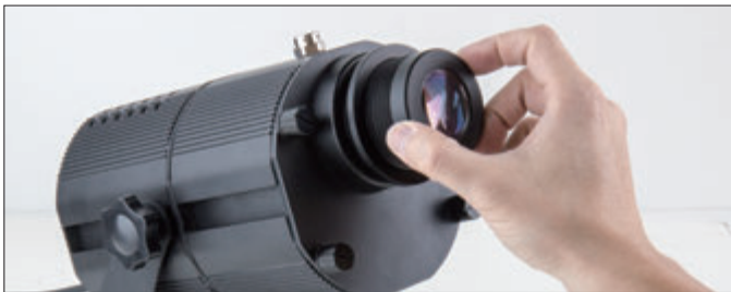
High definition optical focal lens is adjustable by turning clockwise or counter-clockwise to get the clear projection image. Make the inner ring with gasket to contact the housing firmly for waterproof seal.
