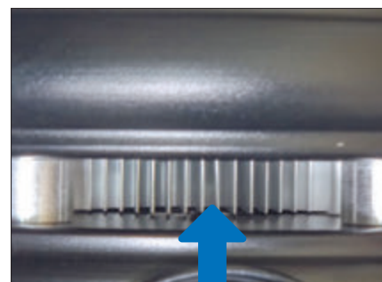
Heat sink for better ventilation.
