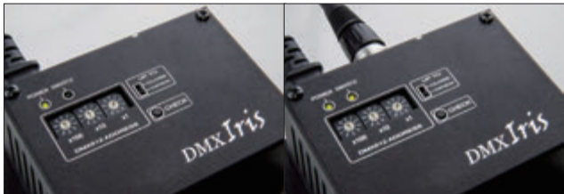
LED lights up while the AC power comes in.
