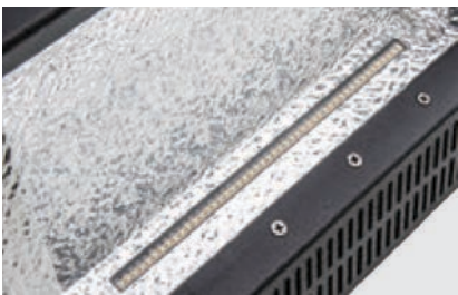
LED light engine consists of 48pcs LED, available with RGBA, 3200K warm white, tunable white (3200K warm white + 6000K cool white), and UV LED at 365nm.
