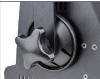
Yoke lock washer provides positive locking; ventilation slot makes the better controls of working temperature.
