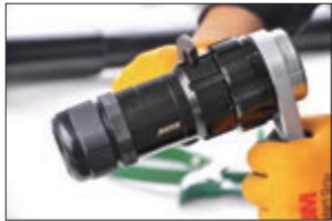
WPC-5219ST and WPC-5219SY spanners helps with tightening the connector.
