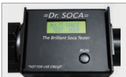
Cable Testing Mode
