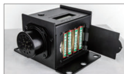
DR.Soca can be used either with 4 x AA Battery.
