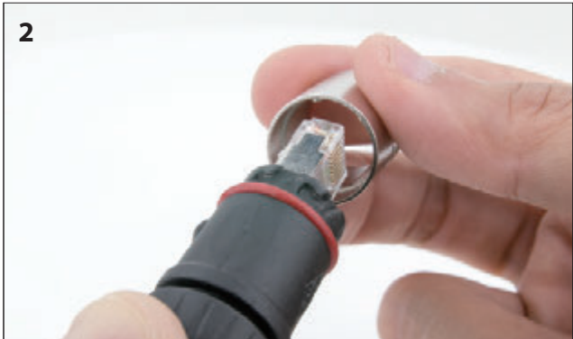
Align the key to the slot.
