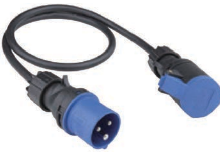
Cable: H07RN-F 3 x 2.5mmsq Connector: 16A 2P+E CEE form (230V)
