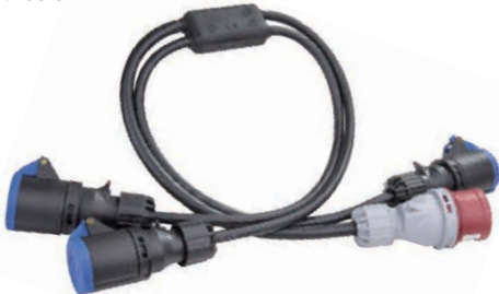
YS-16331-CEE 3-phase Y splitter to three single phase, length 100cm, parallel wired with 16A CEE connectors
