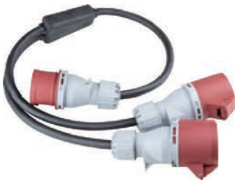
YS-32323-CEE 3-phase Y splitter, fan out to two three phase, length 1M, parallel wired with 32A CEE form connectors
